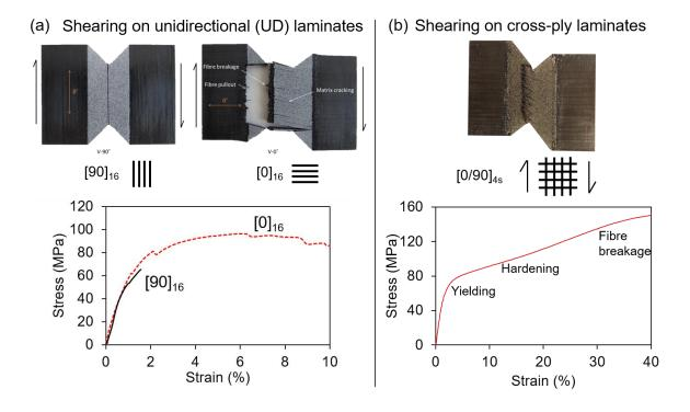
Figure 1. The failure modes and stress-strain curves of V-notched shear tests of AS4/PEKK carbon fibre thermoplastic composites [2]. (a) Shear loading is applied parallel and perpendicular to fibre direction on the unidirectional laminates (b) shear loading is applied on cross-ply laminates.
