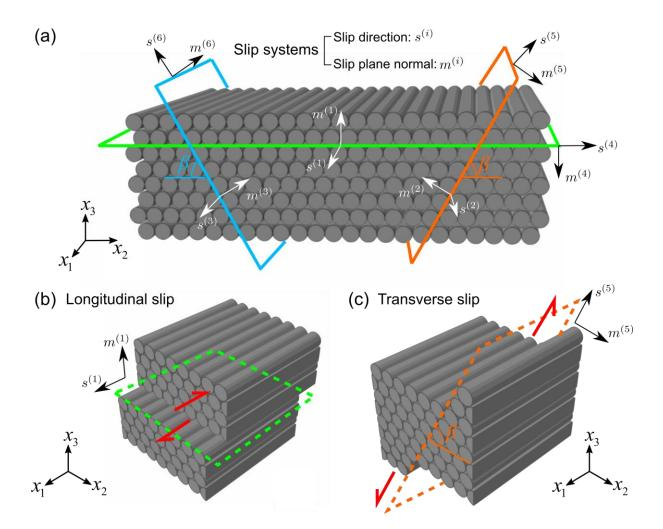
Figure 4. Sketches of (a) six typical slip systems with slip direction  $s^{(\alpha)}$  and slip plane normal  $m^{(\alpha)}$ . (b) The slip system  $(s^{(1)}, m^{(1)})$  in the longitudinal direction and (c) the slip system  $(s^{(5)}, m^{(5)})$  in the transverse direction.
