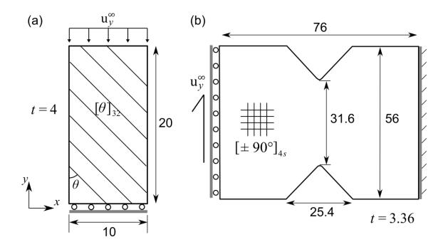
Figure 7. Specimen geometries for (a) IM7-8552 unidirectional composite laminates of different off-axis angle subject to uniaxial compressive loading [3] and (b) AS4-PEKK cross-ply composite laminates subject to shear loading. Note that thickness is denoted by t. All units are in mm.
