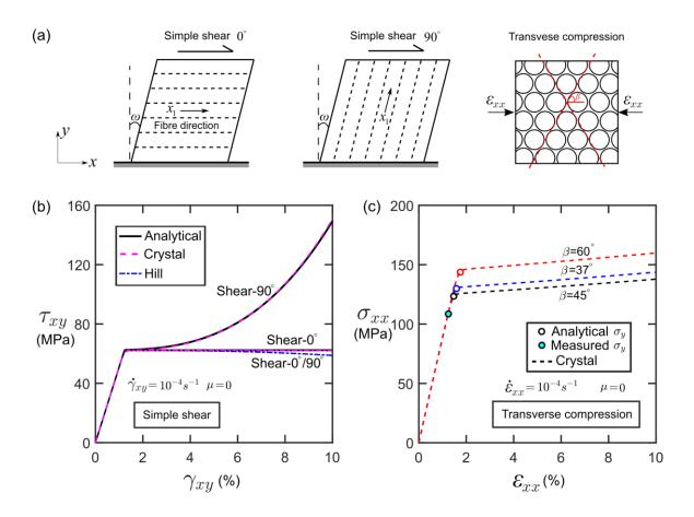
Figure 6. (a) Sketches of boundary conditions: simple shear 0°, simple shear 90°, transverse compressive tests of a unidirectional lamina. (b) Predicted stress-strain curves of simple shear on a unidirectional lamina using the crystal plasticity model and Hill's model. (c) Predicted stress-strain curves of a unidirectional lamina under transverse compression of slip system oriented at  $\beta = 37^\circ, 45^\circ, 60^\circ$  respectively.
